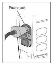
**<u>CAUTION</u>**: Failure to push the connector all the way forward may result in an intermittent connection, and the connector may dislodge, causing a loss of power.
